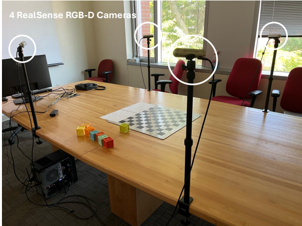
Figure 3. Data collection setup with four Intel D455 RealSense cameras. Camera intrinsics and extrinsics are estimated prior to recording using a checkerboard calibration.
